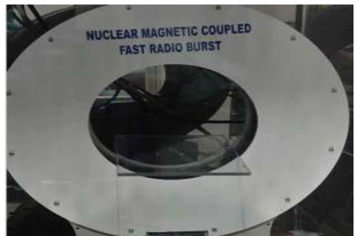
Figure 3: NMCFRB machine for this study: The gantry that delivers the NMCFRB described in the methodology is possible with this specialized device constructed for the purpose. It is designed to hold cell culture plates not exposed in the sham control or exposed in the experimental procedure, and can be place within a CO 2 incubator shown below.
