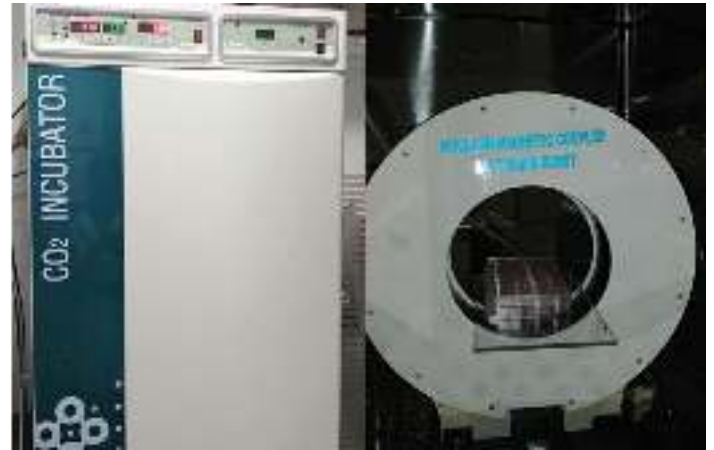
Figure 4: NMCFRB device assembled and placed inside the CO 2 incubator: The machine (not shown in the original size) used to deliver the FRB is placed inside a CO 2 incubator and the experiments entailing the use of two dimension and three dimension cultures described in the methodology was carried out.
