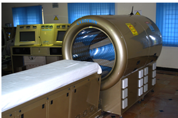
Figure 1A: The CYTOTRON® whole body device. The CYTOTRON-RTE-6040-864GEN (Class IIA Medical Therapeutic Device; developed by Scalene Cybernetics Ltd, Bengaluru, India) is seen in the foreground. The wide-bore gantry houses 864 guns distributed in 9 axes, with each axes bearing 96 guns to deliver RF & MR as per protocol; a moving patient bed and built in device control unit. The central control & command computer for dosimetry planning is seen in the background.
